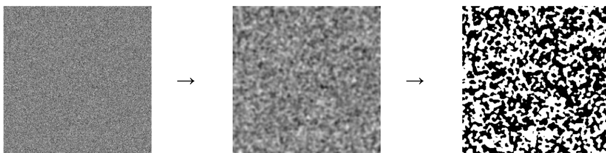
Fig. 1. Synthetic Noisy Microscopy Image → Denoised Image (Gaussian Filter) → Segmentation Mask (Thresholding)
